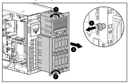
Figure 2-16. Removing the Wide-Ultra hot-plug drive cage assembly
